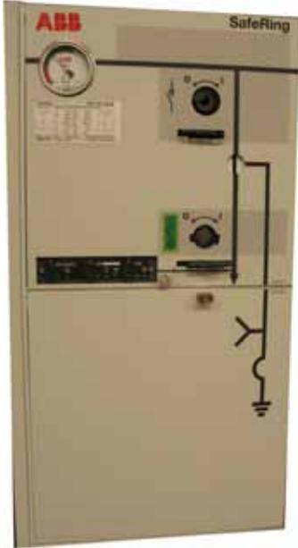
As an option, both C- and De-modules can be equipped with cable test bushings situated behind the lower front cover. This cover can be interlocked against the earthing switch to avoid access to the cable test compartment before earthing switch is in closed position.
